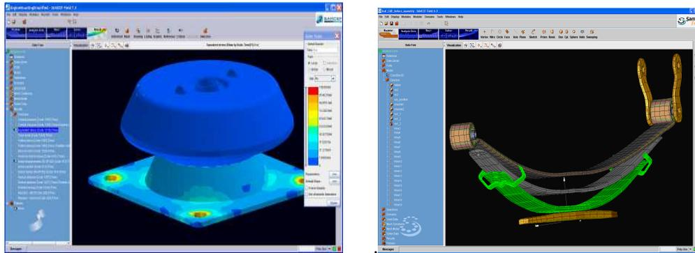
**Figure 1:** Bushing and leaf spring examples having large deformation to take into account
