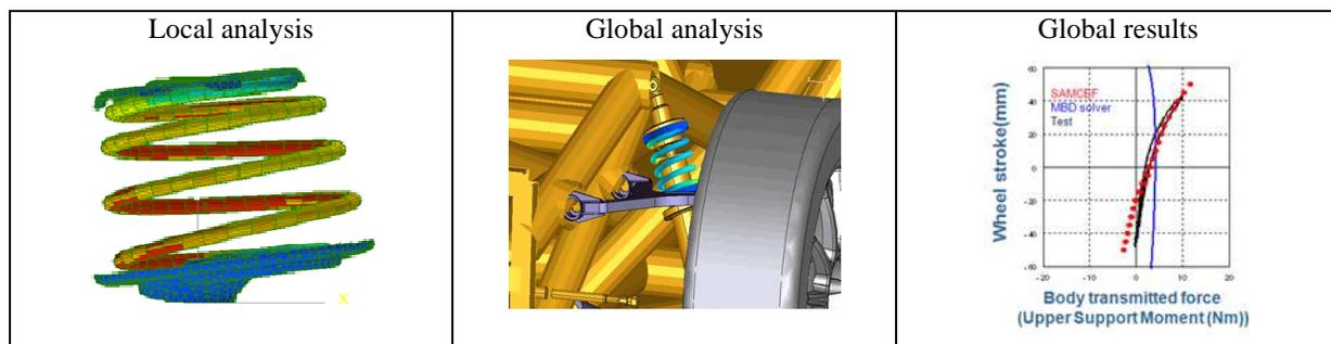
**Figure 2:** Meshed spring included and comparison with classical MBS (Green Propulsion)
