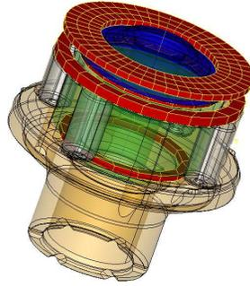
**Figure 5:** Differential managing gears system and contacts with variation of friction (JTEKT Torsen)
