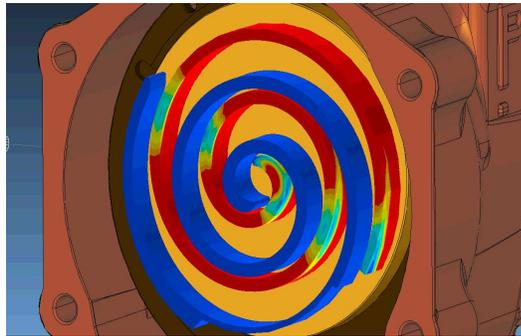
**Figure 8:** Scroll compressor (DENSO)
