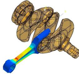
**Figure 3:** Meshed connecting rod inside a rigidly modelled engine
