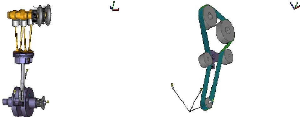
**Figure 4:** Transmission from flexible belt taken into account in MBS (Evolve Powertrains)
